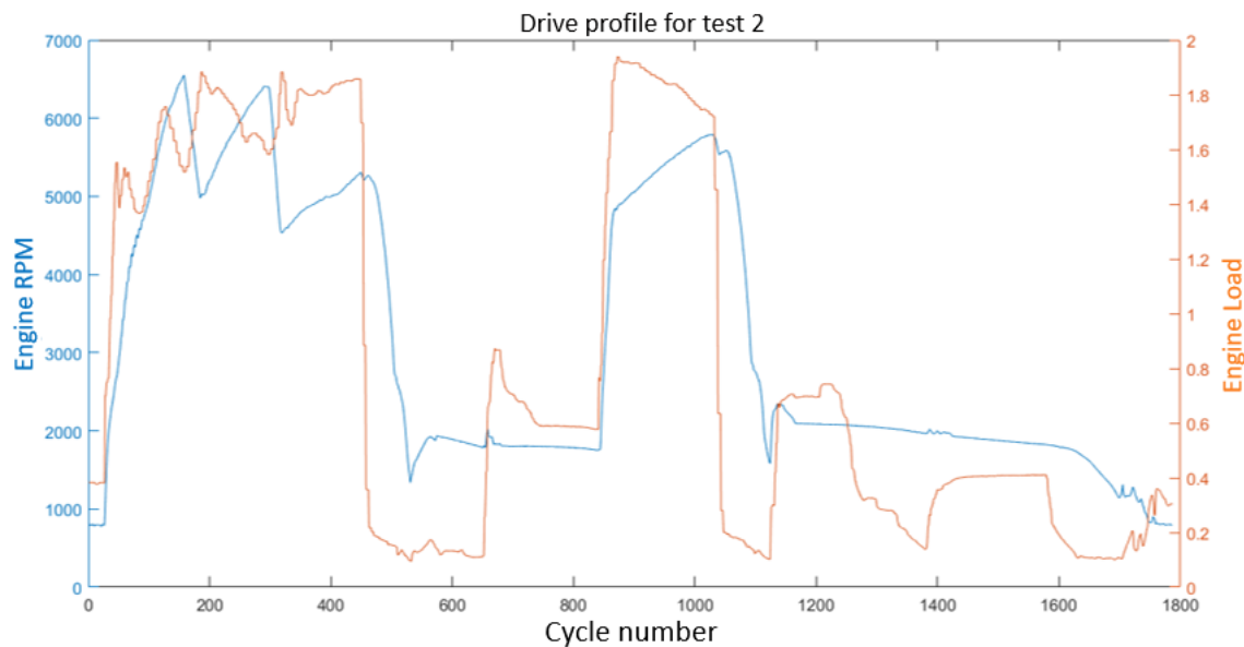
Figure 5.37: Transient drivecycle for evaluating exhaust signatures of low load cycles
